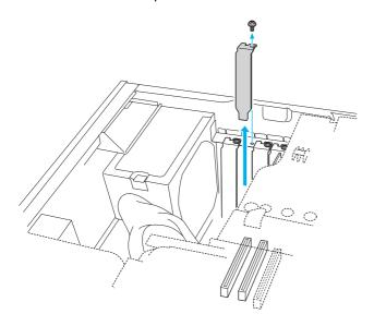
When removing a slot cover, be careful not to damage components on the system board or add-on cards. You may need to temporarily remove add-on cards or other components that may be next to the slot cover you want to remove.
